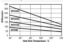
This graph shows the maximum wattage rating for each possible resistor of standard size corresponding to the heat sink temperature. It is assumed that all resistors are equally loaded.
