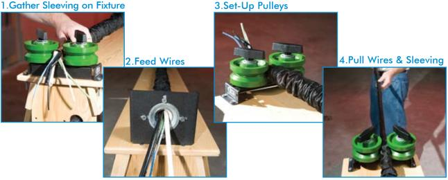
This completely modular system allows production level installation of braided sleeving over wire and cable bundles of virtually unlimited length. The system is simple to set up and interchangeable components accommodate diameters up to 2". For more information about this product contact your Account Representative.
