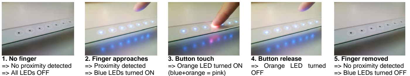
Figure 60 Touch+Proximity Module Operation
