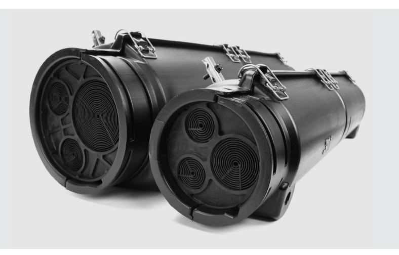
New SLiC fiber closures and terminals are designed for strand-mount FTTH in-line, butt or taut sheath applications. This weather-tight product is a single piece construction that can be installed very easily. The single piece construction permits complete splice access after placement without removal of the closure or terminal from the cable.
