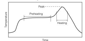
Recommended soldering conditions for flow
