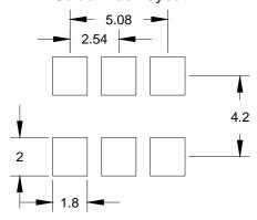
Note: XPRESSO LVDS VCXOs are designed to fit on Industry standard, 6 pad, layouts.
