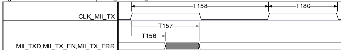
Figure 14-15. MII Interface Output Signal Timing
